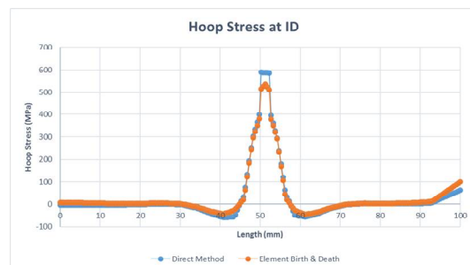
Figure 27 Hoop Stress along the Inner diameter (225°)
